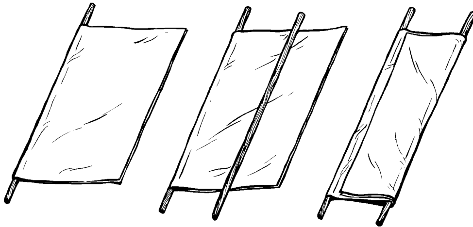
Figure 9-8. Litter made with blanket and poles.
