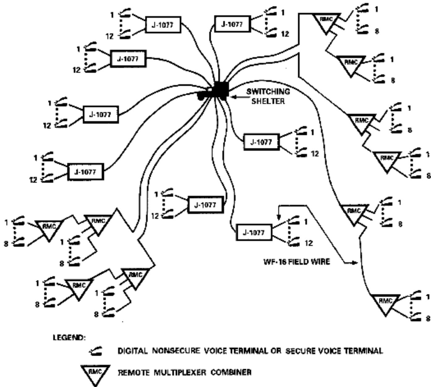
Figure 3-6. Large extension, node switchboard interface.
