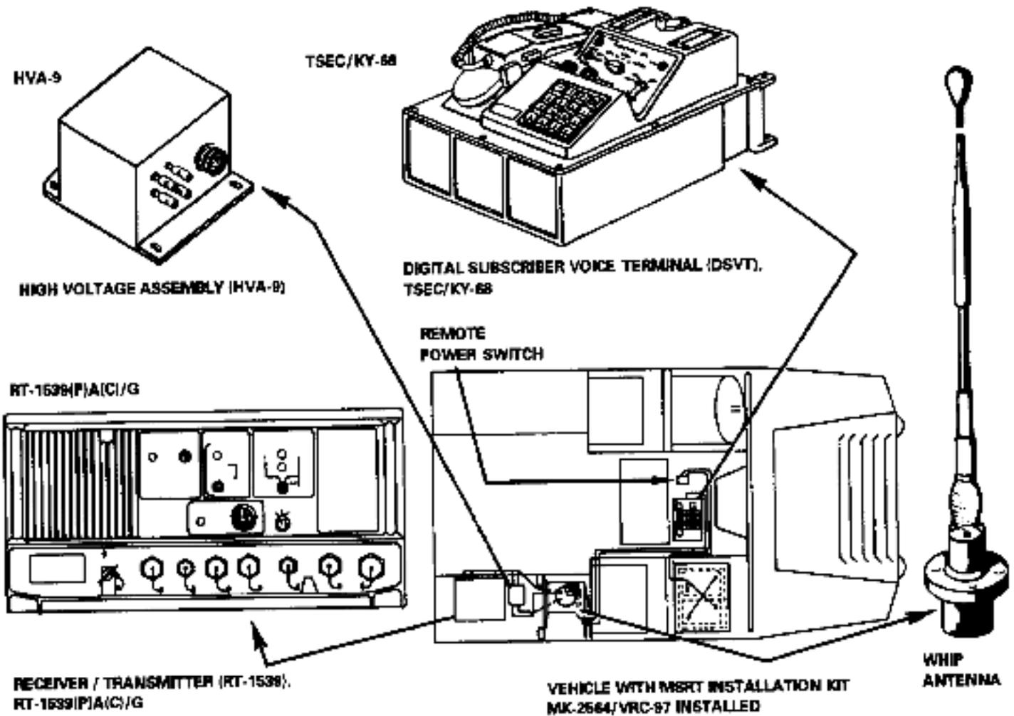
Figure E-10. Typical mobile subscriber radio/telephone installation.
