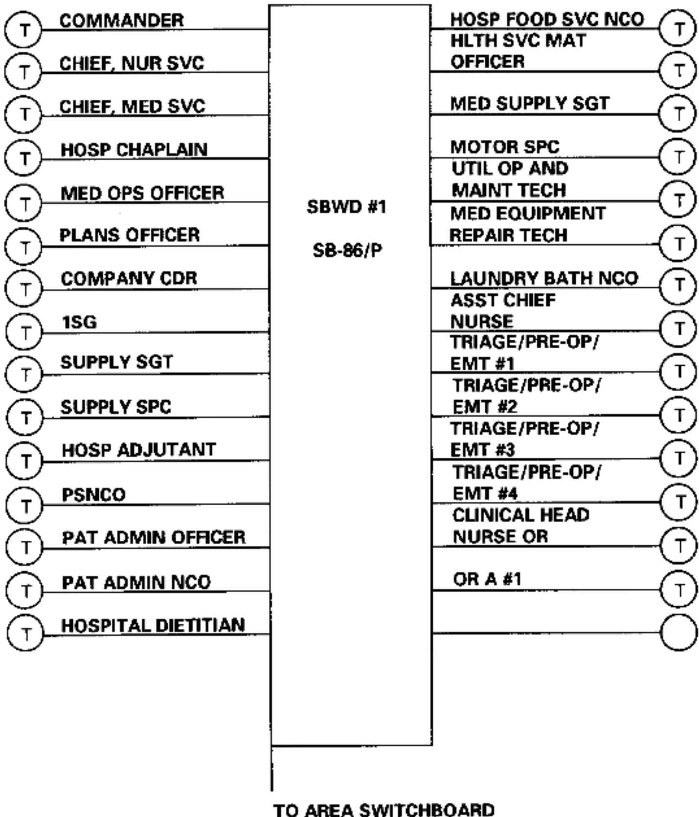
Figure 3-7. Wire net diagram, CSH, switchboard 1.
