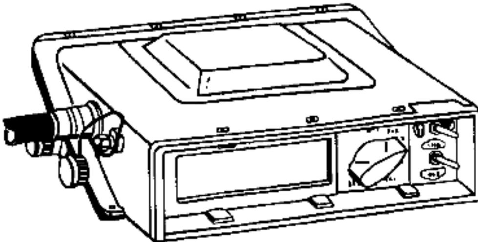
*Figure E-9. Precision lightweight global positioning system receiver.*
