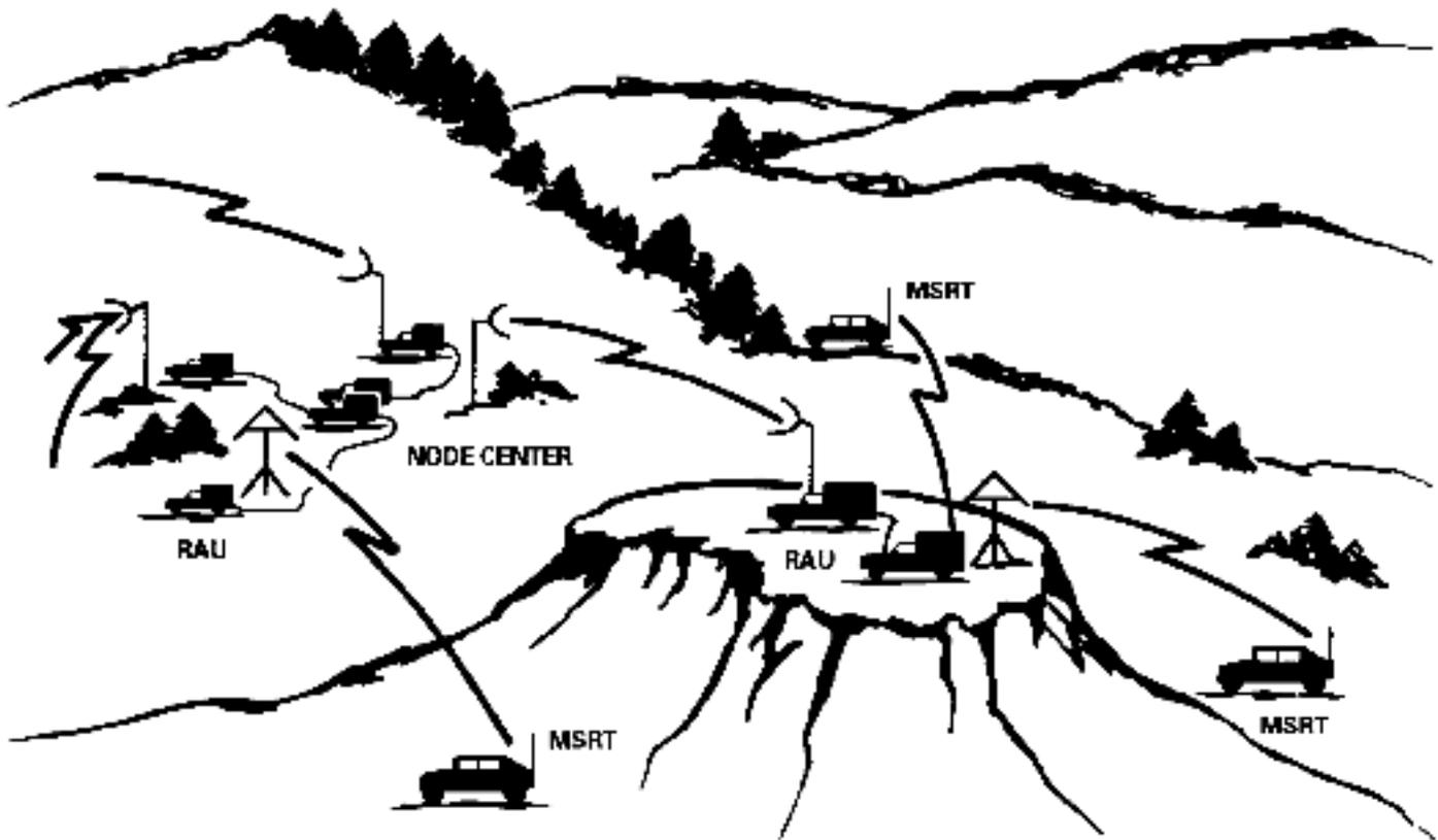
*Figure 3-1. Typical mobile subscriber connectivity.*
