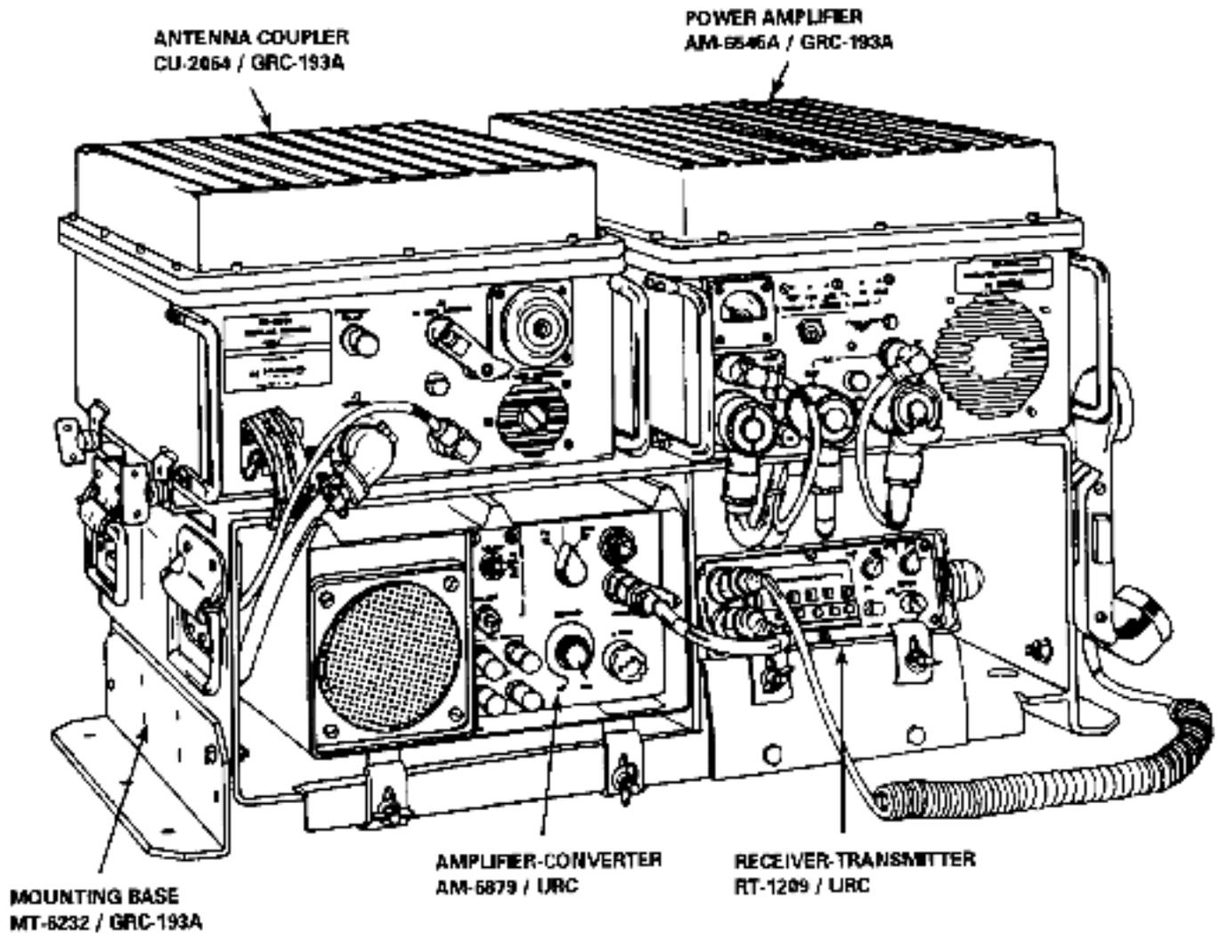
Figure E-4. Improved high frequency radio.
