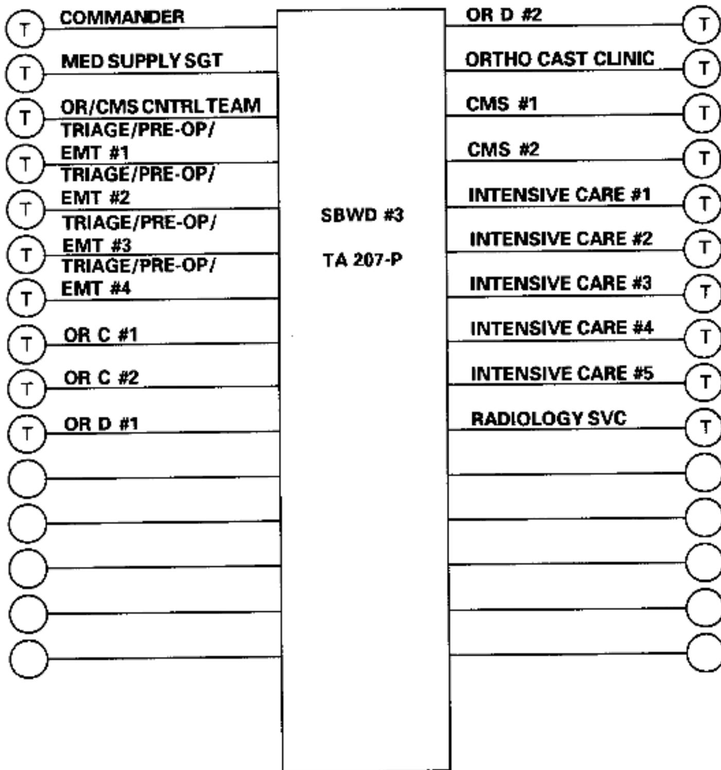
**NOTE: ONE OF THE SB-86/Ps IS AUGMENTED WITH A TA 207-P (SIGNAL ASSEMBLY SWITCHBOARD) TO PROVIDE 30 ADDITIONAL SWITCHBOARD LINES.**
