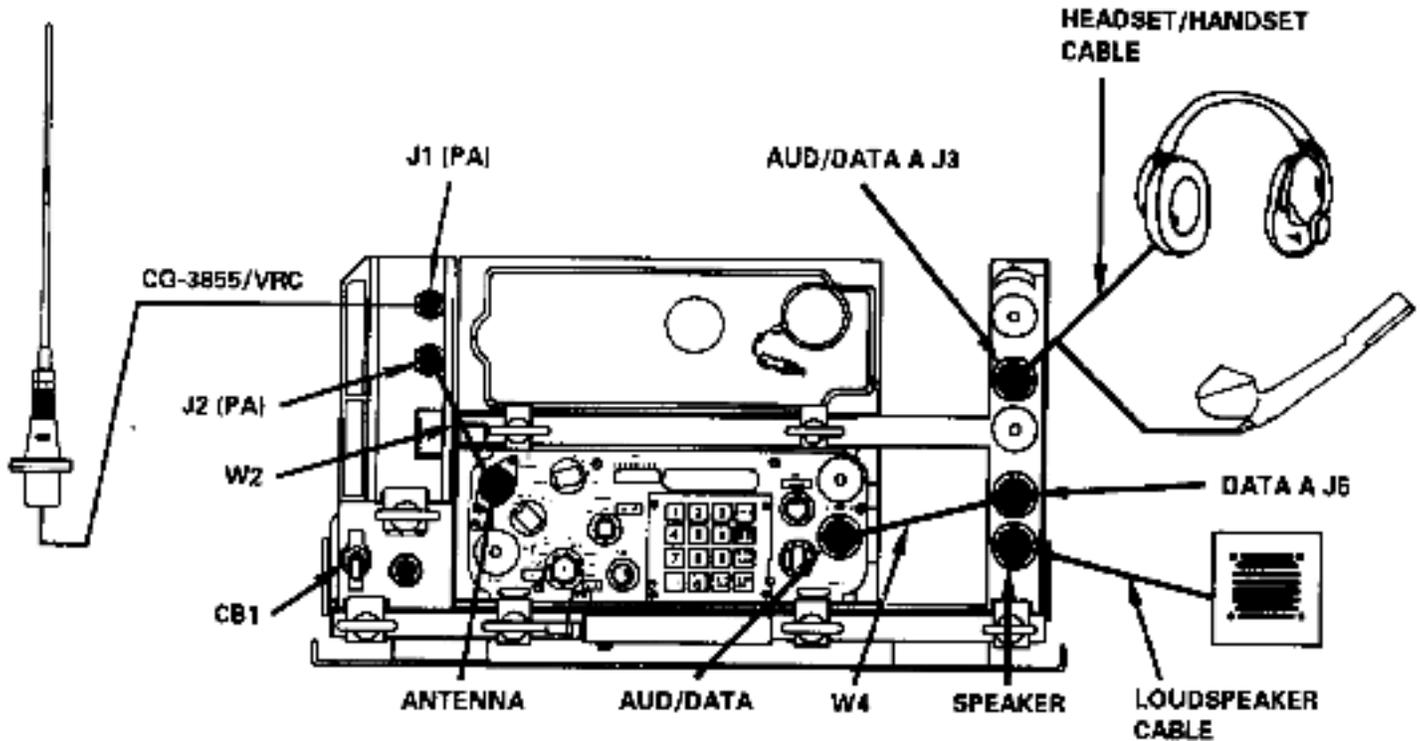
Figure E-3. Vehicular long-range radio, AN/VRC-90A.
