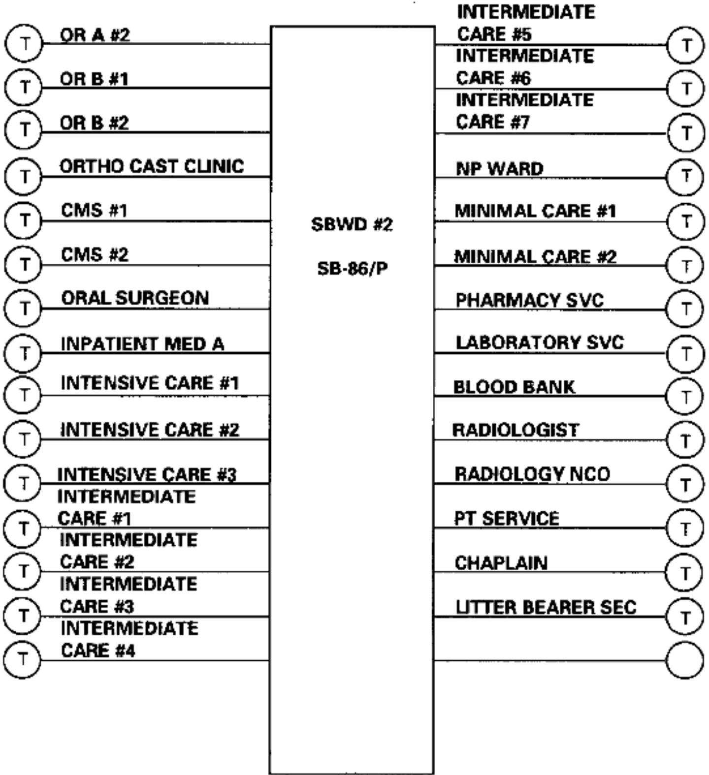
Figure 3-8. Wire net diagram, switchboard 2.
