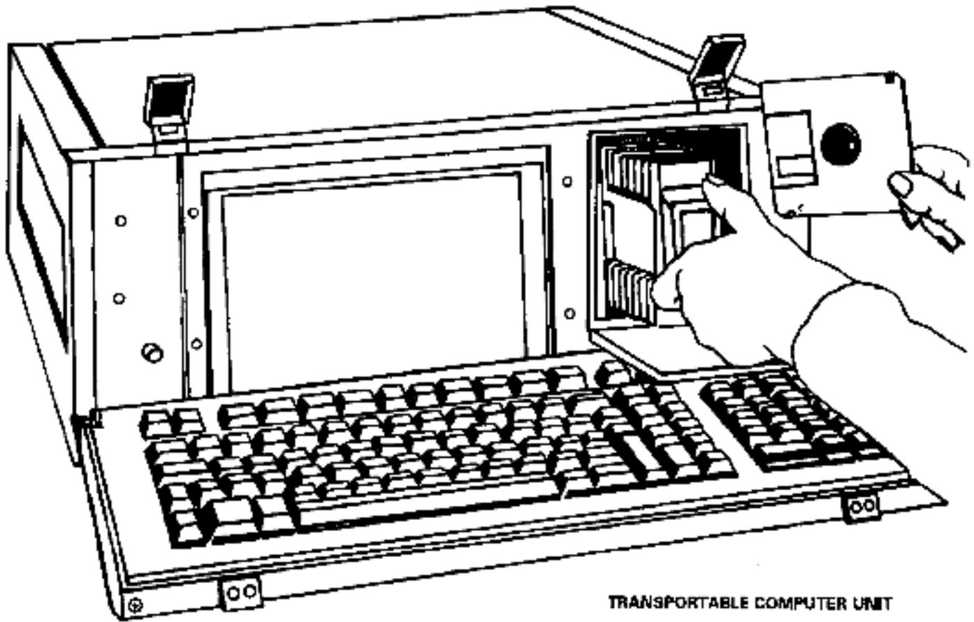
*Figure E-7. Medical transportable computer unit.*
