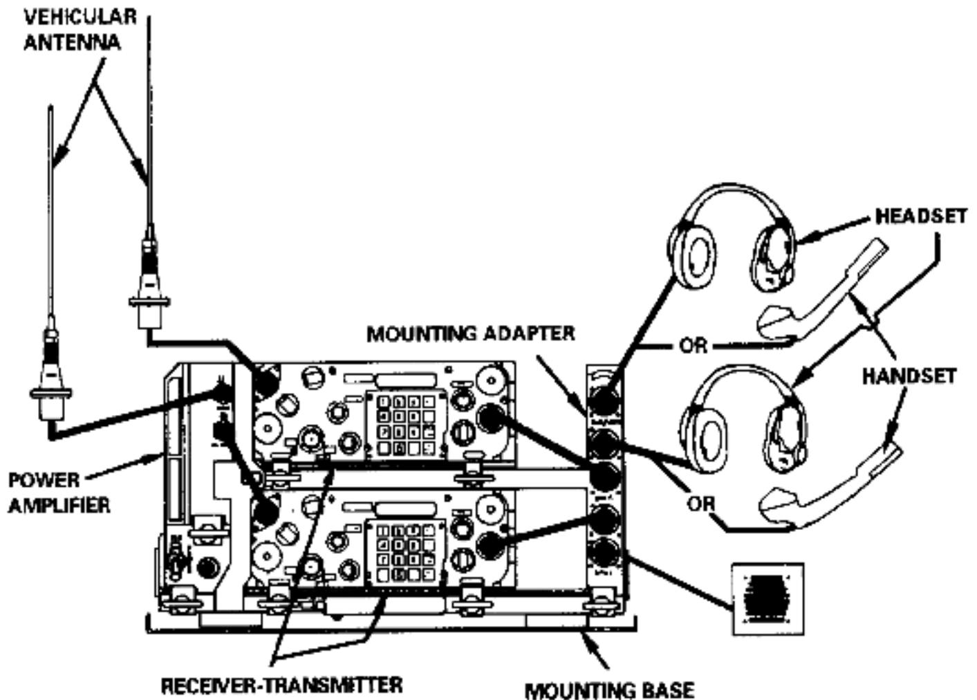
*Figure E-2. Vehicular long-range/short-range radio, AN/VRC-89A.*
